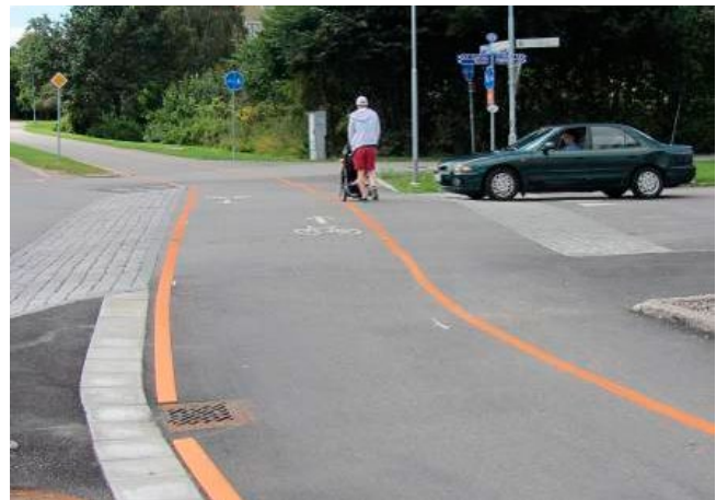
Junction with continuous cycle lane
